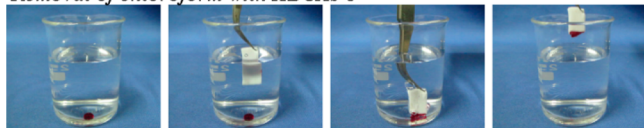
Figure 9. Removal of a red-colored plant oil spill (15 \mu\text{L} ) from water with the slices (ca. 20 \times 8 \times 2 ) of (top row) HBCAs and (middle row) BCAs; (bottom row) removal of chloroform from the bottom of water with the slice of HBCAs.
